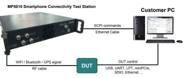
VSA/VSG engines run on the MP5010 Tester Mass-production software runs on the customer's PC
