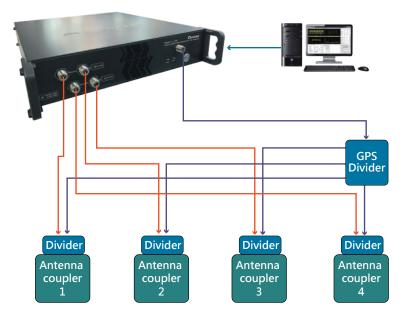
Using the WIFI/GPS parallel test, combined with the hardware of the MP5010, implement 4-port multi-site parallel test with single satellite GPS solution, which increases the test speed of the production line by more than three times
